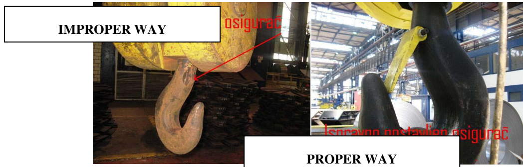
Figure 4: Crane hook without fuses and with fuses
