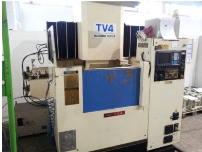
Figure 3. Machining center with safety barrier
