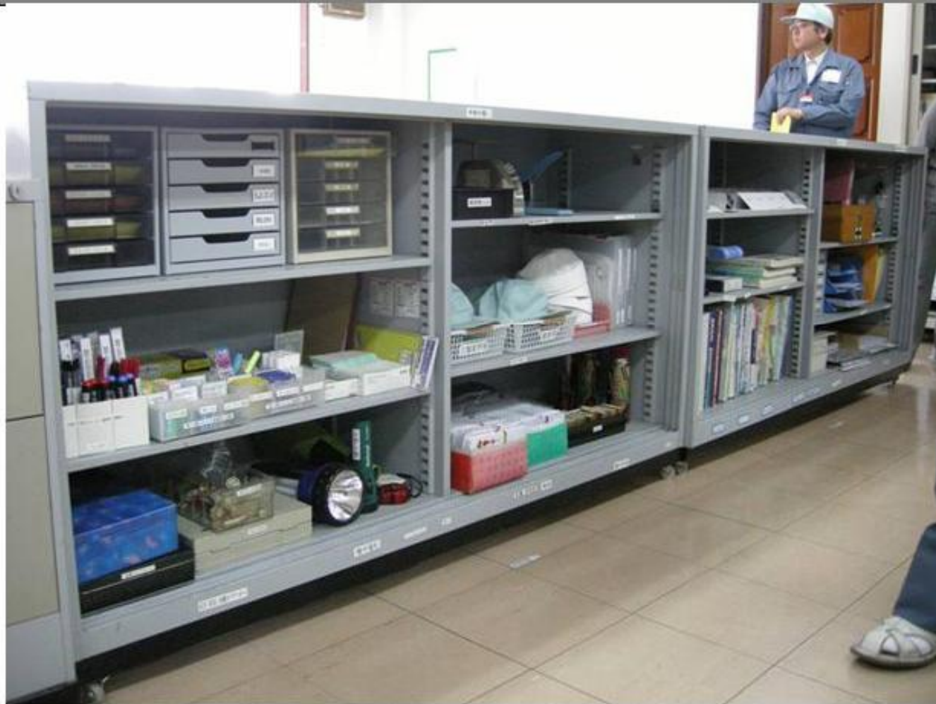
5S – all material identified and in its place. In the furniture, the wheels to facilitate moving.
