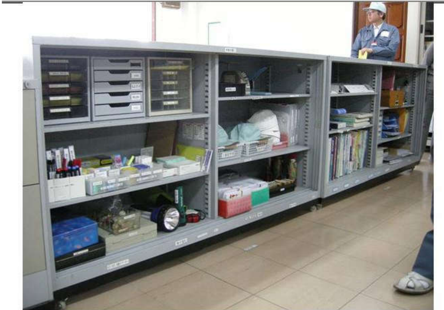
5S – all material identified and in its place. In the furniture, the wheels to facilitate moving.
